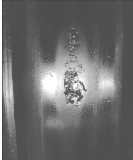
**Figure 2: Intermediate stage of shell growth from small skid flat.**
