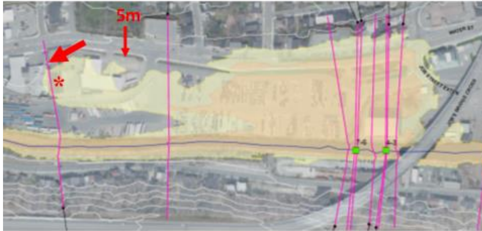
Figure 4-13 Portion of Waterford River Current Floodplain Boundary; Red arrow identifies Transect WR 1-10; Hospital shown as *
