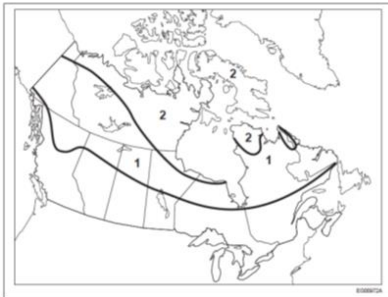
Figure 2-25 Map of Permafrost Zones in Canada (Source: Figure K6, Commentary K NBC Structural Commentary, Part 4, Division B 2015).
