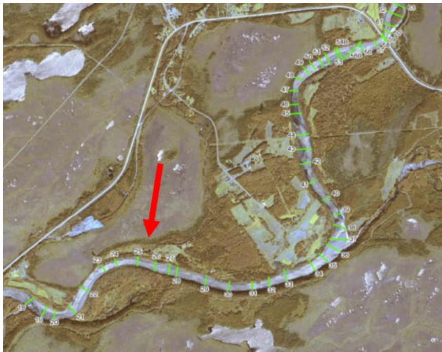
Figure 2-4 Harry's River; Cross Sections overlaid on aerial imagery. Cross Section 25 identified by red arrow (source: Hydrotechnical Study of Stephenville Crossing/Black Duck Siding, 2012)
