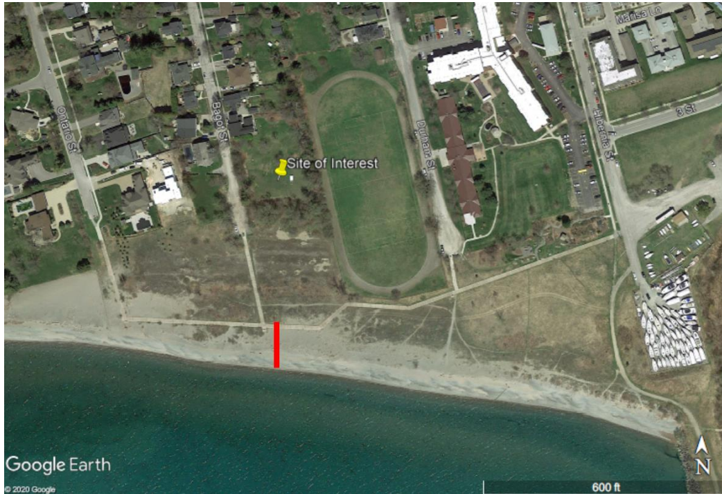
Figure 2-42 Lake Ontario Site of Interest, red line is 30 m setback of the dynamic beach
