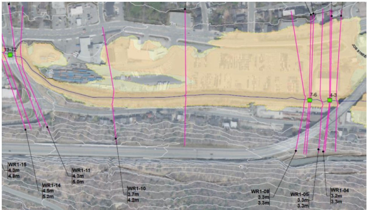
Figure C-8 1:20 and 1:100 AEP Floodlines Waterford River, NL Future Conditions
