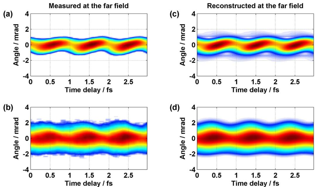
**Figure 3. Reconstructing the far-field pattern of an isolated attosecond pulse.** (a,b) Far-field pattern measured as a function of time delay for photon energy of 30 eV (a) and 60 eV (b). (c,d) The reconstructed far-field pattern obtained by using the phase retrieval algorithm for the photon energy of 30 eV (c) and 60 eV (d).
