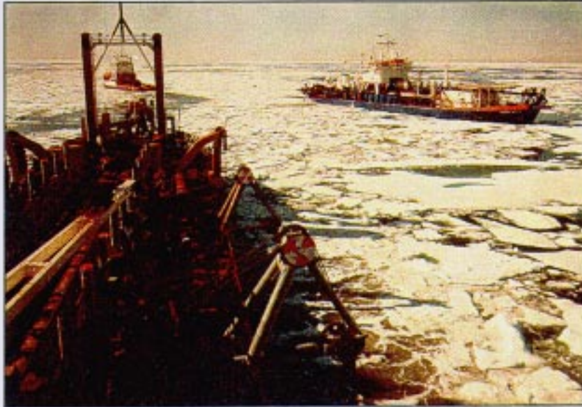
Figure 5.4: Variable concentrations of first year ice hampered the dredging activities that were associated with the construction of the Amauligak I-65 subcut and berm. Ice management support was provided by BeauDril's Arctic Class IV icebreakers which proved very effective in allowing continued dredging activities when significant ice was present.
