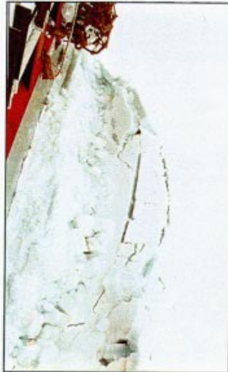
Figure 3.8: Typical examples of buckling. The upper figure shows creep buckling while the lower figure shows flexural buckling that was common at higher ice interaction speeds.
