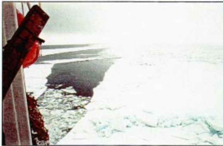
Figure 3.10: Typical examples of large scale fractures propagating out from the Molikpaq's ice interaction front. The top photo shows a number of cracks that in this case were associated with bending ice failures against floating rubble debris adjacent to the caisson wall, while the lower photo shows a crack that formed off one of the caisson's corners and has opened into a small lead. Often, cracks were observed to form at the corners between the Molikpaq's long and short faces and propagate out into the oncoming ice cover.
