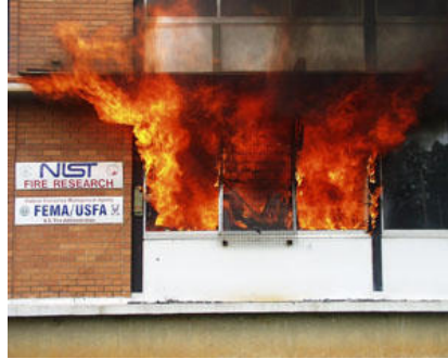
Figure 2: An example of flashover in experiments, from [11].
