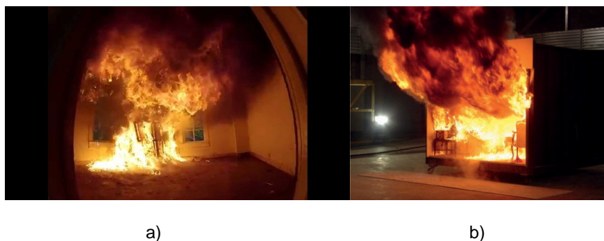
Figure 1: Examples of flashover. a) A flashover captured on GoPro, from [5]. b) Fire development of ceiling layer that shows flashover happening, from [6].
