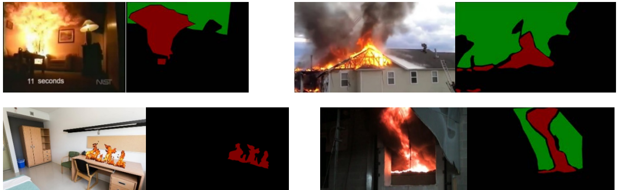
Figure 12: Samples and their annotations (R: flame, G: smoke) from the FS Segmentation dataset. The Upper left image pair is Christmas Tree tests from NIST. The upper right one is image pair from a Fire rescue video posted on YouTube [49]. The lower left image pair is synthetic images generated in this study using Blender. The lower right image pair is from the NRC PRF-07 test.
