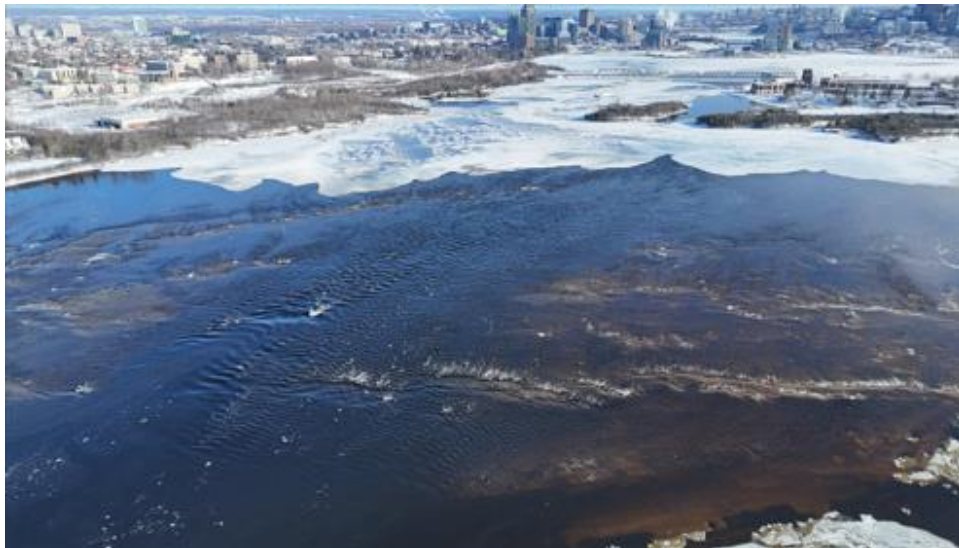
Figure 14: Looking downstream at the Ottawa River, between the cities of Gatineau (left) and Ottawa (right). This site displays the extensive development of anchor ice (light-brown zones), which remained in place for several weeks. Where they come close to the water surface, white water is present. Photo: NRC.
