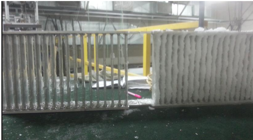
Figure 13: Frazil ice adhesion to two grids. Under the same flow conditions and with similar frazil concentrations, a difference was observed in how the rectangular (right) and foil-shaped (left) grids became clogged. The variation is attributed to differences in the local velocity fields around the bars. Scale: the grids are about one meter in height. Photo: NRC.
