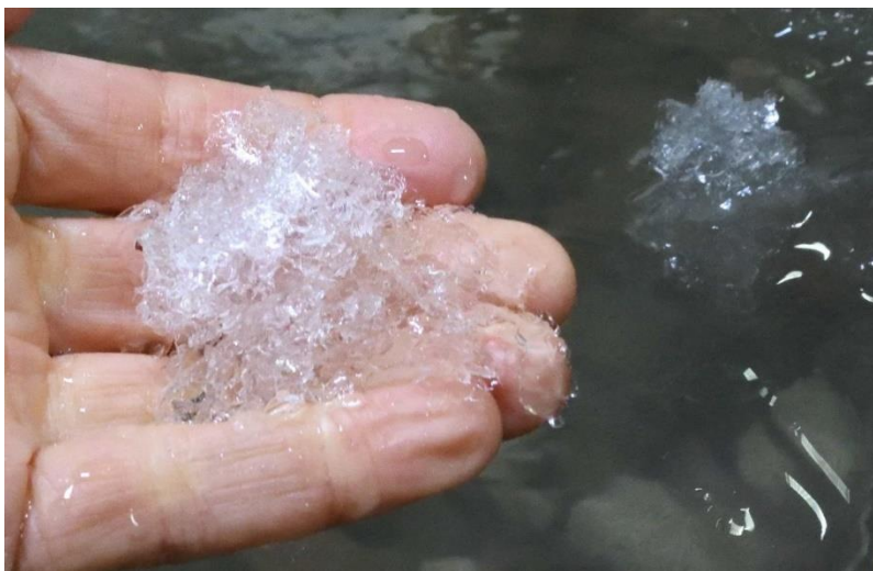
Figure 11: Frazil ice crystals also from a laboratory setup. Photo: NRC.
