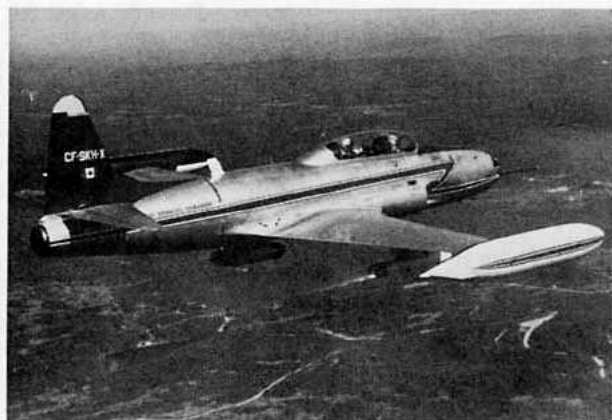
FIG. 1a. T-33 aircraft with gust probe on nose and flare racks underneath wings.
