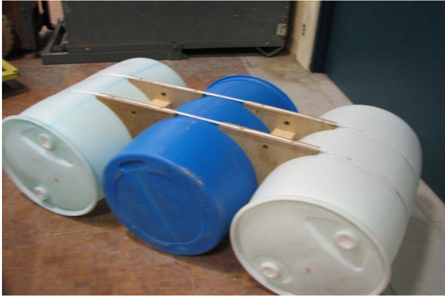
Figure 4 – 3-barrel obstacles used in the simulated ice field
