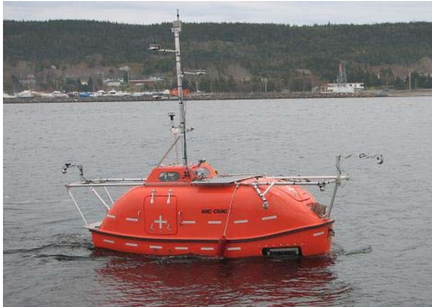
Figure 5 - Lifeboat during VAST field trials showing exterior modifications
