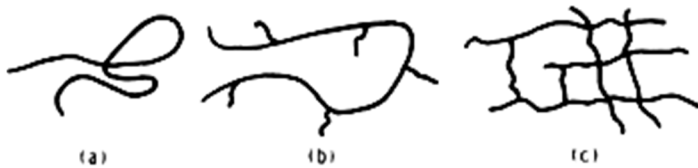
Figure 2. Schematic Representation of Polymer Molecules: (a) Linear (b) Branched (c) Cross-linked
