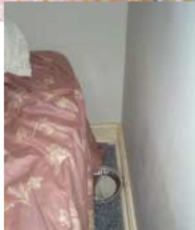
Figure 18. A queen-size bed ignited with a small amount of diesel in the fuel pan.
