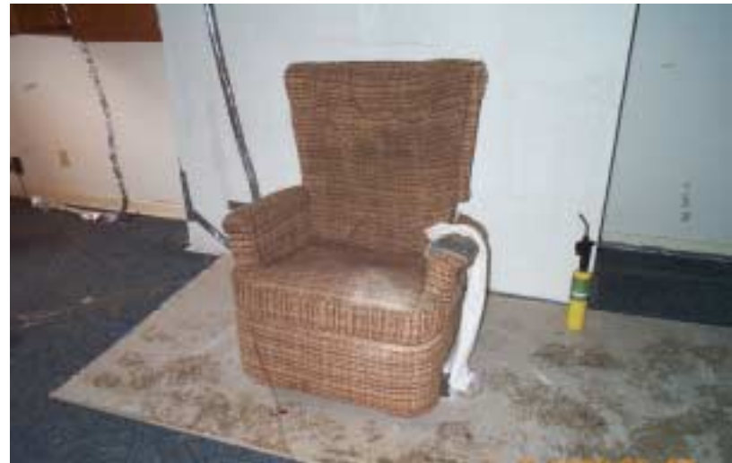
Figure 13. Chair directly under exposed pipes, with thermocouples installed on the chair, unprotected pipe and in the cavity of open wood joist and with diesel dripped onto the arm, cloth and fuel pan (Test 2).
