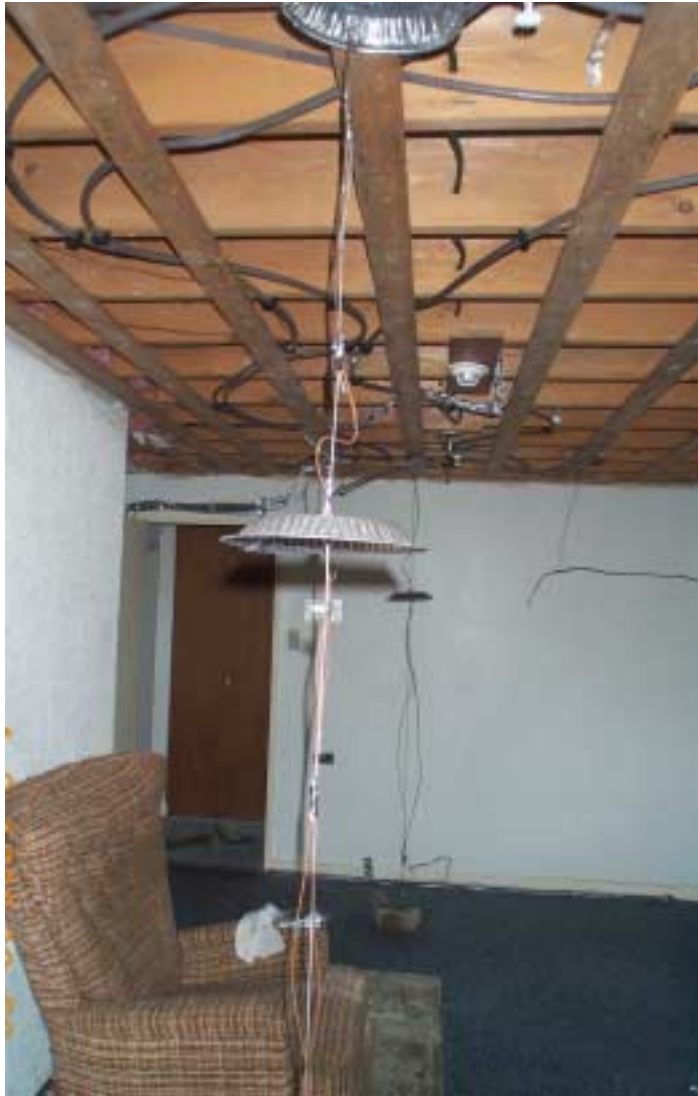
Figure 13. Chair directly under exposed pipes, with thermocouples installed on the chair, unprotected pipe and in the cavity of open wood joist and with diesel dripped onto the arm, cloth and fuel pan (Test 2).
