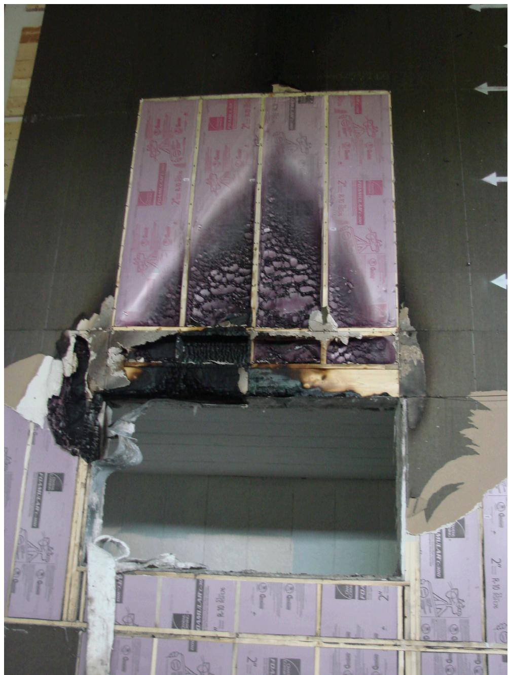
**Figure 13. Wall Sample after Fire Exposure.**
