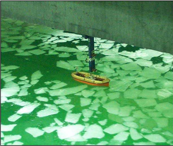
Fig. 1. Resistance test of TEMPSC design in pack ice using a tow pole
