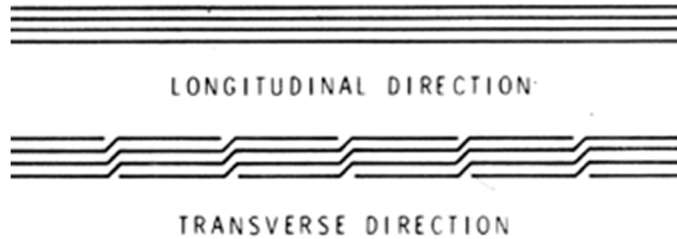
Figure 1. Sections through 4-ply membrane.
