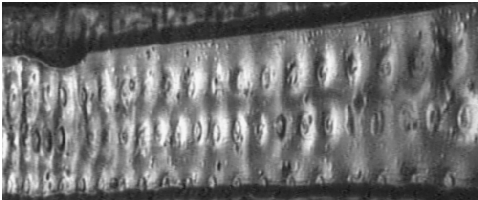
Figure 24b). D Sight inspection results for lap joint 349C. De-painted, SolidHi.
