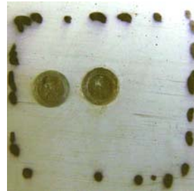
M43 w/ head rivet popped out
