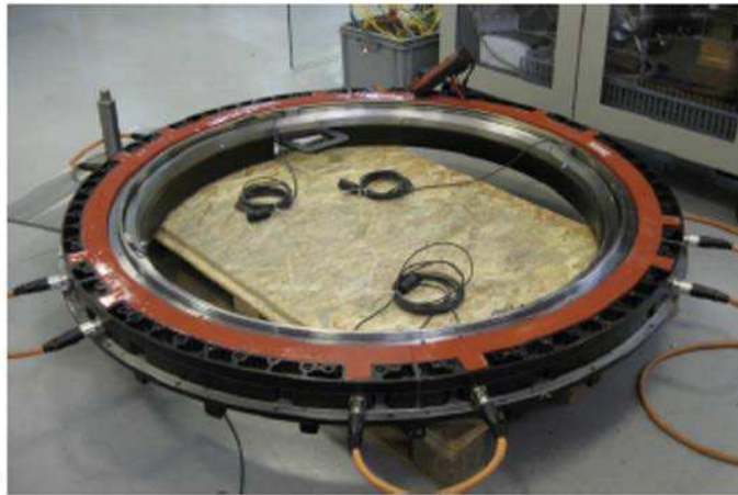
Figure 71: InRo – Example of a dedicated, integrated, low-voltage torque motor, made by PHASE MOTION CONTROL, for rotator application.
