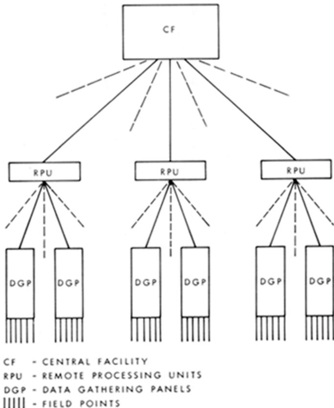
Figure 1. Block diagram for Class B systems.
