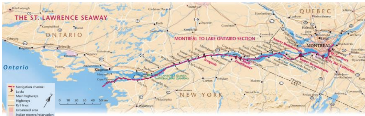
Figure 9: The St. Lawrence Seaway between Lake Ontario and Montreal (Jenish, 2009). The name of the seven locks is indicated in red font – in the upstream direction: St. Lambert, Côte Ste Catherine, Lower and Upper Beauharnois, Snell, Eisenhower and Iroquois.
