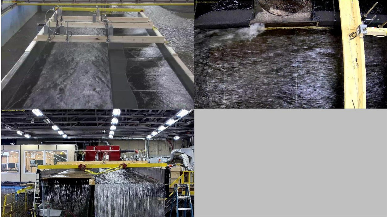
Figure 23. Image capture from the test videos for 2022-7-11_test001, 2.5% Grade, 2.0% cross-slope, single curb inlet (S22)
