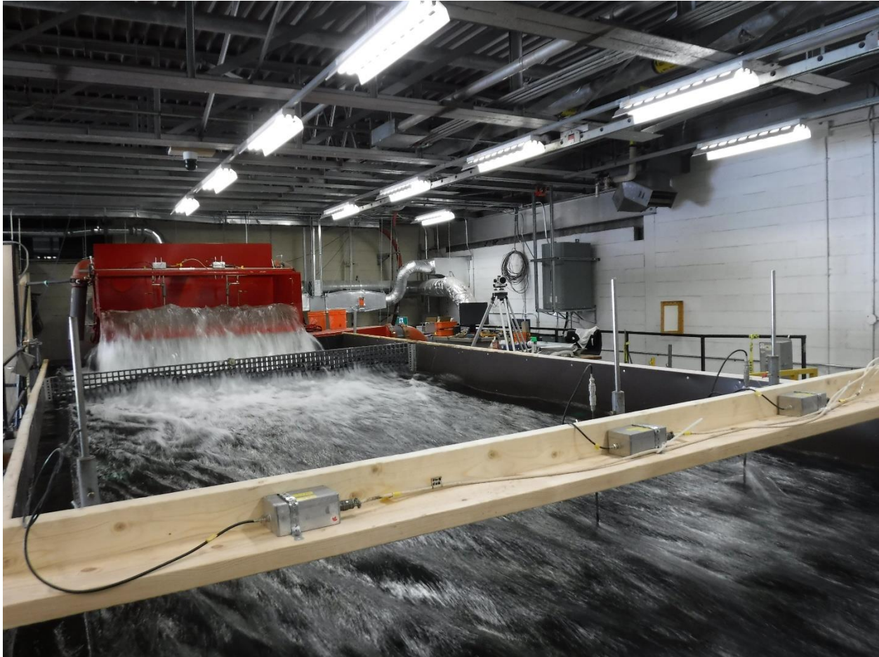
Figure 24. Water flowing from the head tank to the roadway, high flow conditions
