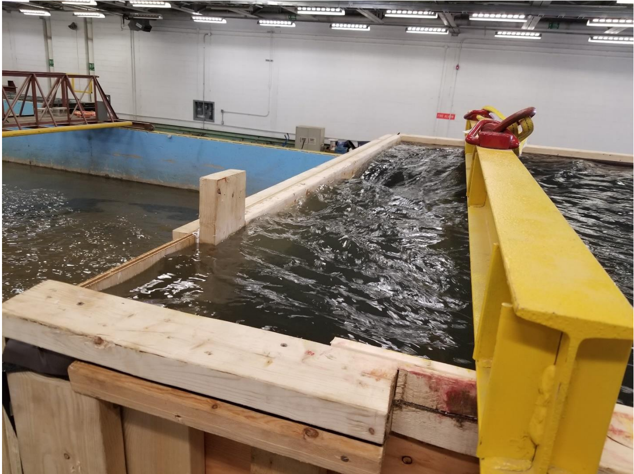
Figure 4. Blocked roadway for ponding test
