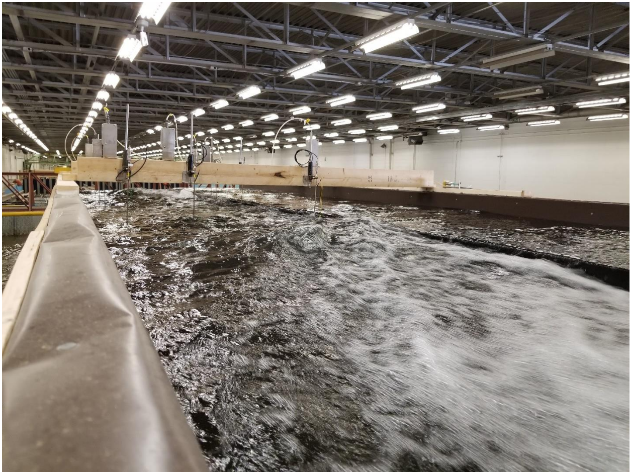
Figure 30. Photo taken during 2022-7-8_test005A, 0.5% grade, 2.0% cross-slope, single curb inlet (S22), incident water depth of 17.1 cm.
