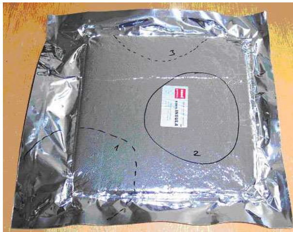
Figure 44: Sample preparation for the permeability measurements.
