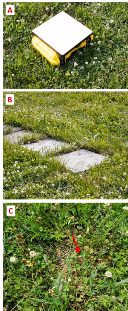
Figure 6. Target materials used for comparison. (A) InfraGold panel atop a plastic storage box, used as a platform to keep the surface debris free. (B) Concrete patio stones with three heat flux sensors (black squares on the concrete slab—as also indicated in Figure 4 label E) from which temperature was derived. The left-most sensor did not stay adhered to the surface and therefore, the data were not used. (C) In-canopy temperature sensor T1 (located with the red arrow) within the living and detritus vegetation canopy. The in-canopy temperature sensors (T1 and T3) were positioned at a height of approximately 2–3 cm above the soil.
