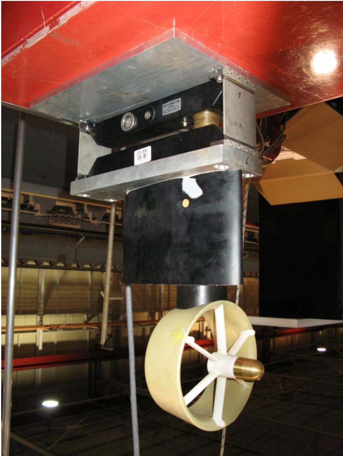
Figure 4: Nozzle and Stator Assembly on 1-Component Balance
