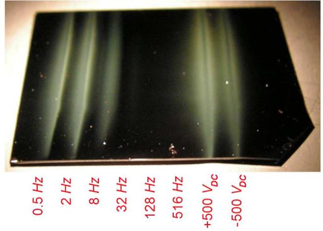
**Fig. 5.** Mechanism of droplet precipitation. Aerosol deposition performed under alternating voltage (500 V amplitude) at various frequencies (0.5–516 Hz) is compared with deposition at constant voltage. Concentration and duration were 2  $\mu\text{g/mL}$  and 90 s, respectively. Sample dimension is 25  $\times$  30  $\text{mm}^2$ , approximately.
