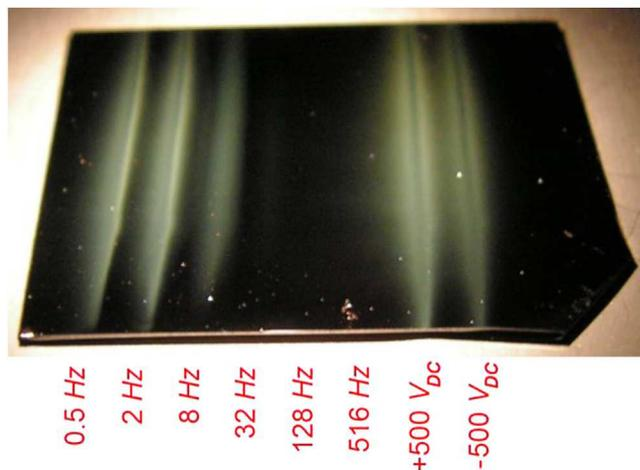
**Fig. 5.** Mechanism of droplet precipitation. Aerosol deposition performed under alternating voltage (500 V amplitude) at various frequencies (0.5–516 Hz) is compared with deposition at constant voltage. Concentration and duration were 2 μg/mL and 90 s, respectively. Sample dimension is 25 × 30 mm<sup>2</sup>, approximately.
