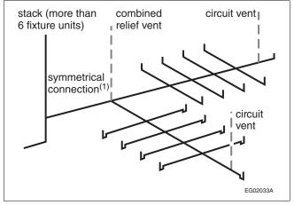
Figure A-2.5.3.1.-F Example of circuit venting described in Sentence 2.5.3.1.(5) Note to Figure A-2.5.3.1.-F:
