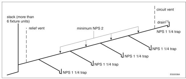
Figure A-2.5.3.1.-K Example of circuit venting described in Sentence 2.5.3.1.(9) Note to Figure A-2.5.3.1.-K:
