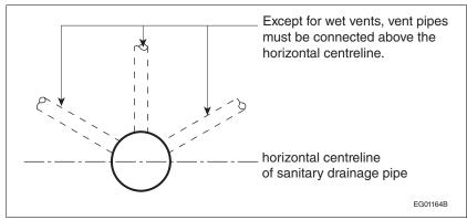
Figure A-2.5.6.2.(2) Vent pipe connections
