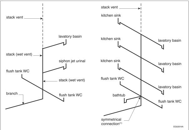
Figure A-2.5.2.1.-B Example of wet venting described in Clause 2.5.2.1.(1)(c) Note to Figure A-2.5.2.1.-B:
