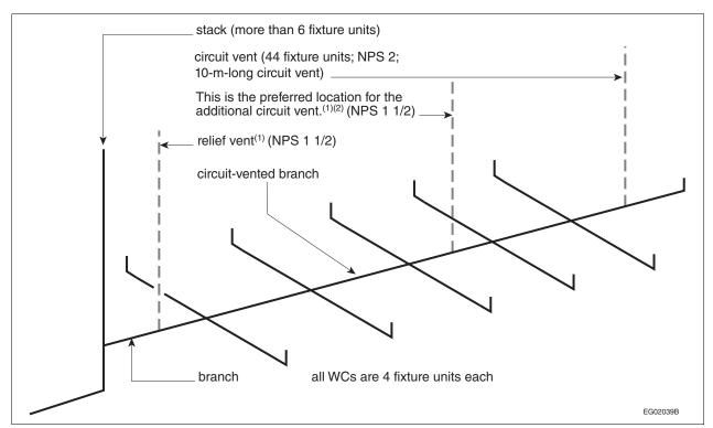
Figure A-2.5.3.1.-L Example of circuit venting described in Sentence 2.5.3.1.(10) Notes to Figure A-2.5.3.1.-L:
