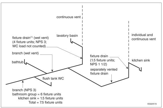
Figure A-2.5.2.1.-E Example of wet venting described in Clause 2.5.2.1.(1)(f) Note to Figure A-2.5.2.1.-E:
