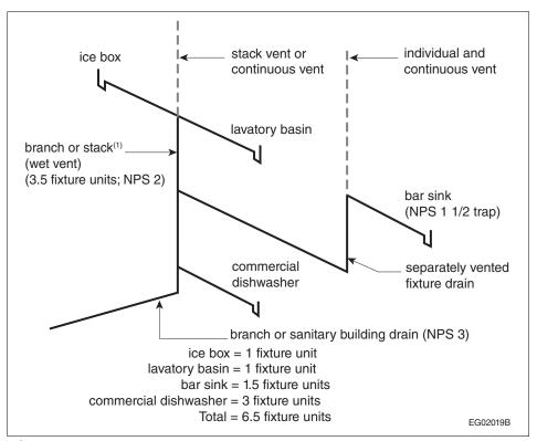
Figure A-2.5.2.1.-G Example of wet venting described in Clause 2.5.2.1.(1)(f) Note to Figure A-2.5.2.1.-G:
