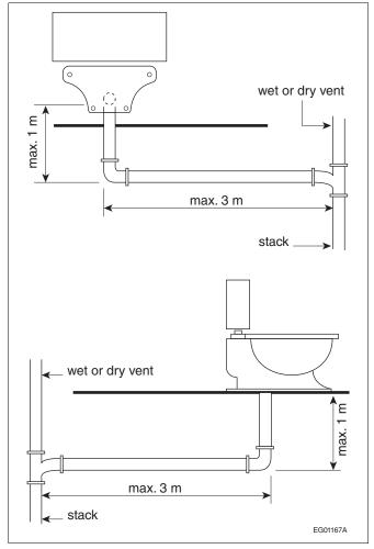
Figure A-2.5.6.3.(3) Length of water-closet fixture drain Note to Figure A-2.5.6.3.(3):
