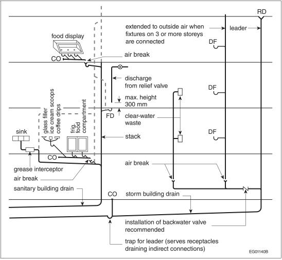
Figure A-2.4.2.1.(1)(a)(ii) and (e)(vi) Indirect connections
