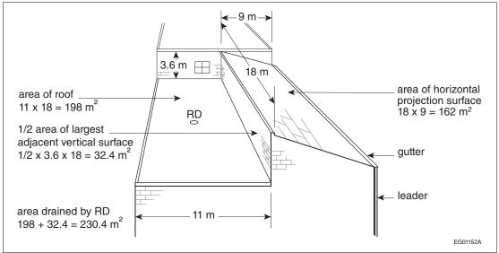
Figure 1-1 Storm drainage areas (example 1)
