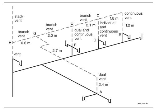
Figure A-2.5.8.3. and 2.5.8.4.-A Lengths to be considered when sizing branch, continuous, dual and individual vent pipes Notes to Figure A-2.5.8.3. and 2.5.8.4.-A:
