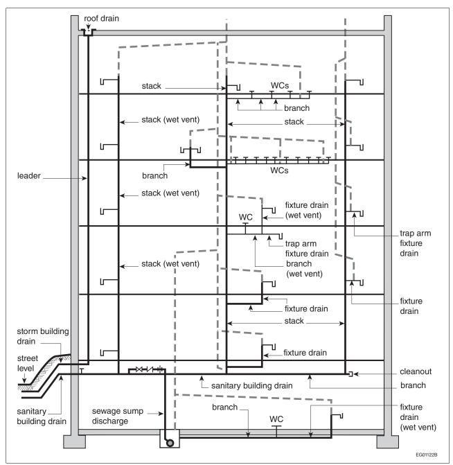
Figure A-1.4.1.2.(1)-F Drainage system
