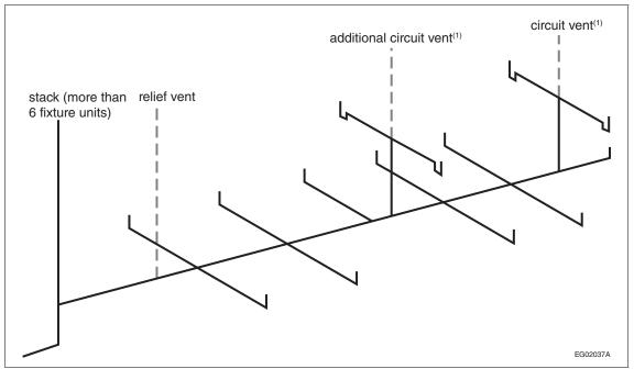
Figure A-2.5.3.1.-J Example of circuit venting described in Sentence 2.5.3.1.(8) Note to Figure A-2.5.3.1.-J:
