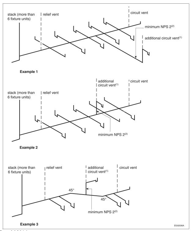
Figure A-2.5.3.1.-I Example of circuit venting described in Sentence 2.5.3.1.(7) Notes to Figure A-2.5.3.1.-I:
