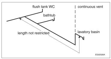
Figure A-2.5.2.1.-M Example of wet venting described in Clause 2.5.2.1.(1)(k)
