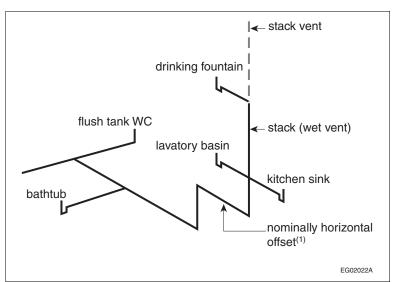
Figure A-2.5.2.1.-I Example of wet venting described in Clause 2.5.2.1.(1)(i) Note to Figure A-2.5.2.1.-I:
