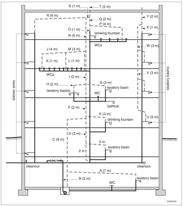
Figure A-2.5.8. Sizing of a venting system
