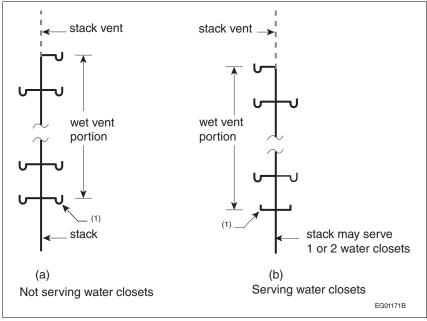
Figure A-2.5.8.1.(2) Sizing of wet vent systems Note to Figure A-2.5.8.1.(2):
