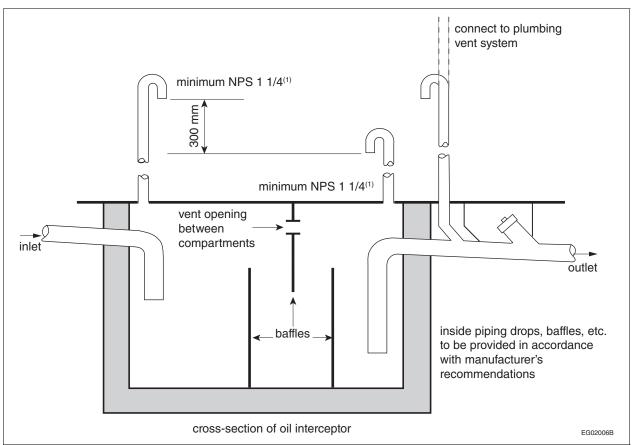
Figure A-2.5.5.2. Venting of oil interceptors Note to Figure A-2.5.5.2.:
