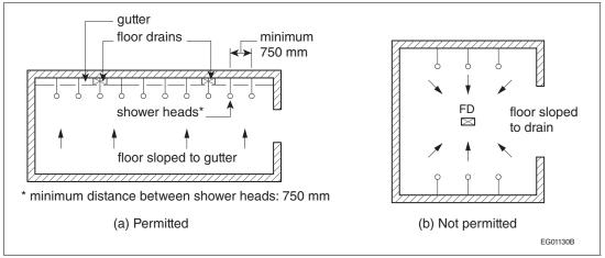
Figure A-2.2.2.3.(3) Shower drainage (plan view)
