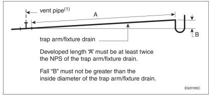
Figure A-2.5.6.3.(1)-A Vent connection
