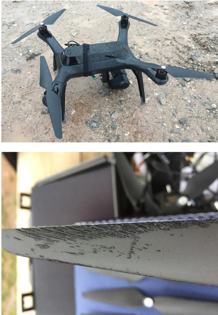
**Figure 12. Ice accretion on the Solo quadcopter.**
