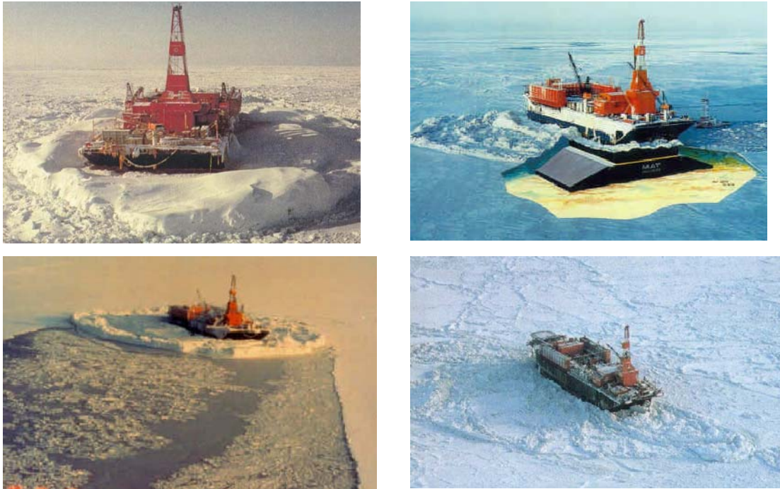
Figure 4.13: Views of the SSDC and its ice pad in winter pack ice conditions in the Canadian Beaufort (left), and as deployed in the Alaskan Beaufort Sea with its MAT (right).
