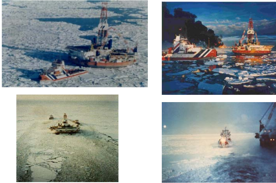
Figure 4.17: Views of the Kulluk and support icebreakers operating in managed ice conditions.
