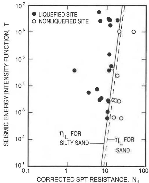
FIG. 8. Correlation of seismic energy intensity function with corrected SPT resistance for silty sand sites from the Chinese data (Xie 1984).
