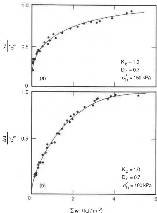
FIG. 3. Typical laboratory test results on Fujian medium sand: (a) triaxial tests; (b) torsional tests.
