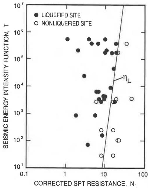
FIG. 6. Correlation of seismic energy intensity function with corrected SPT resistance from the data of Seed *et al.* (1975).
