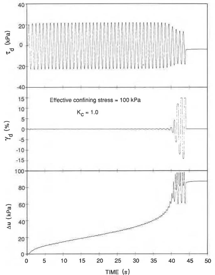
FIG. 2. Typical stress ( $\tau_d$ ), strain ( $\gamma_d$ ), and pore pressure ( $\Delta u$ ) plots of a cyclic torsional test.
