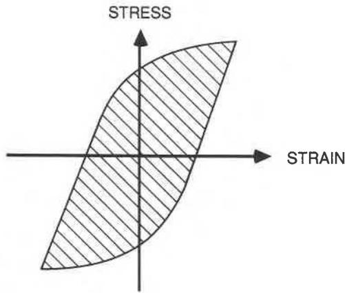
FIG. 1. Hysteretic loop of the soil under cyclic loading.
