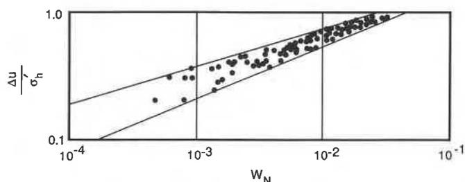
FIG. 5. Normalized excess pore pressure  $\Delta u/\sigma'_h$  vs. normalized dissipated energy  $W_N$  on a log-log plot.
