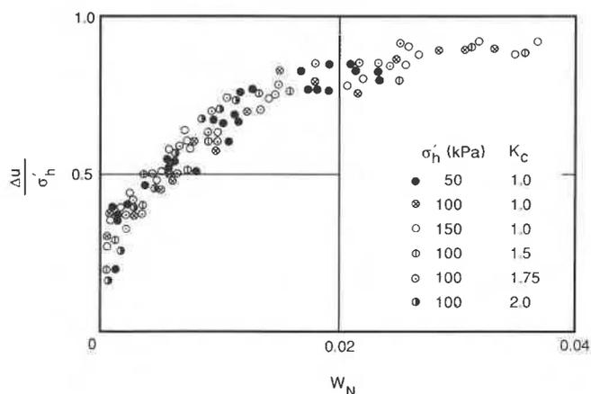
FIG. 4. Normalized excess pore pressure  $\Delta u/\sigma'_h$  vs. normalized dissipated energy  $W_N$ .
