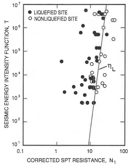
FIG. 7. Correlation of seismic energy intensity function with corrected SPT resistance for sand sites from the Chinese data (Xie 1984).
