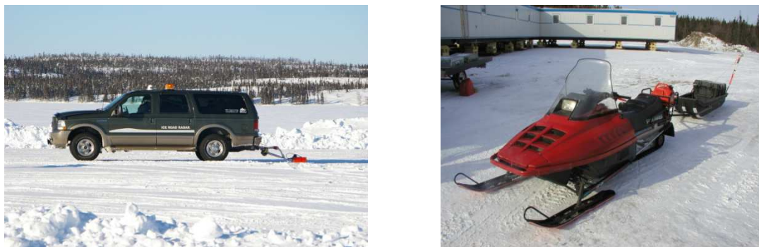
Figure 3: A ground penetrating radar (GPR) system, pulled by a light vehicle (left) or a snowmobile (right), is used to conduct high density ice, thereby closely monitoring ice thickness.
