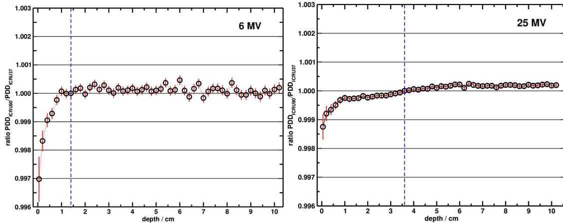
**FIGURE 1:** Ratios of Elekta Precise PDD curves for 6 MV and 25 MV photon beams for a 10 cm  $\times$  10 cm field and an SSD of 100 cm. The vertical dashed line indicates the position of the maximum dose,  $D_{\text{max}}$ . The value at 10 cm depth can be used as an indicator for any relative variation in the beam quality specifier,  $\%dd(10)$ .
