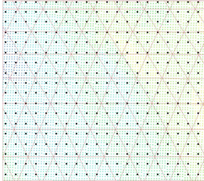
Figure 9 - Definition of the coarser bathymetric set of points, derived from the high density data
