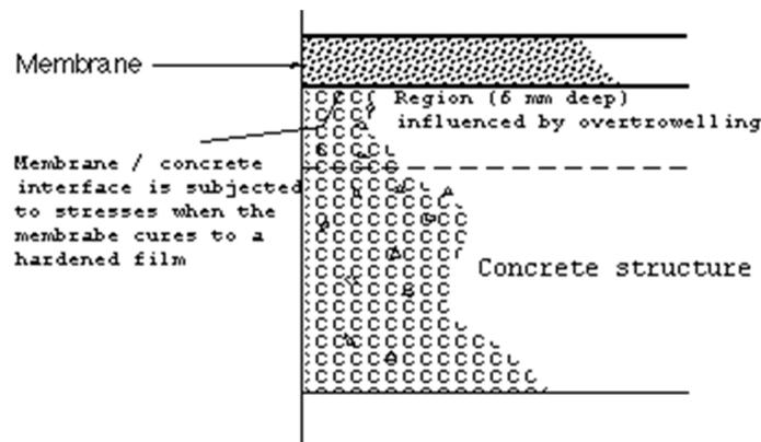
**Figure 2.** Elements of a coating system for concrete
