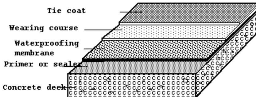
**Figure 1.** Cross-section showing the layer of an elastomeric membrane system on a parking deck
