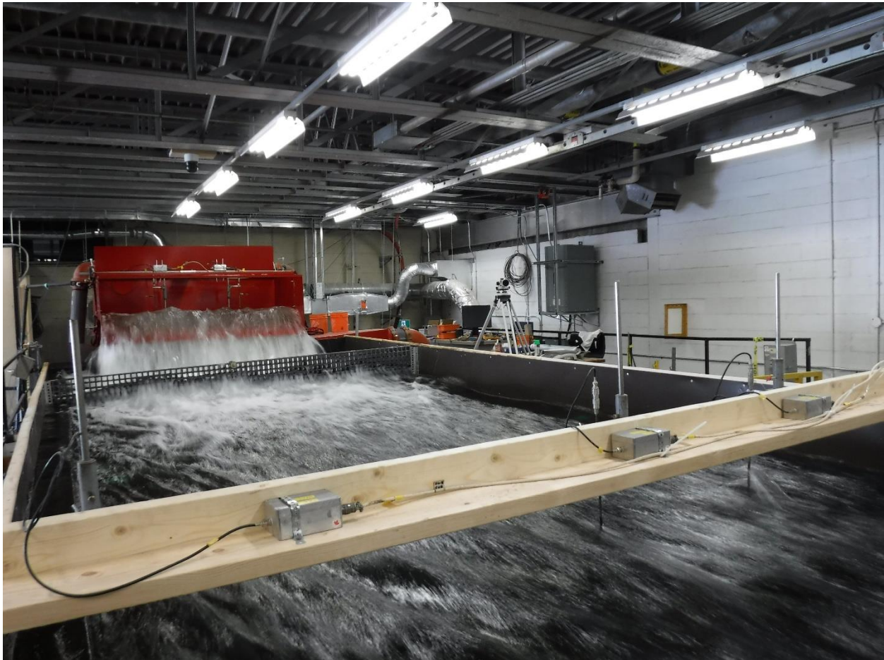
Figure 26. Water flowing from the head tank to the roadway, high flow conditions
