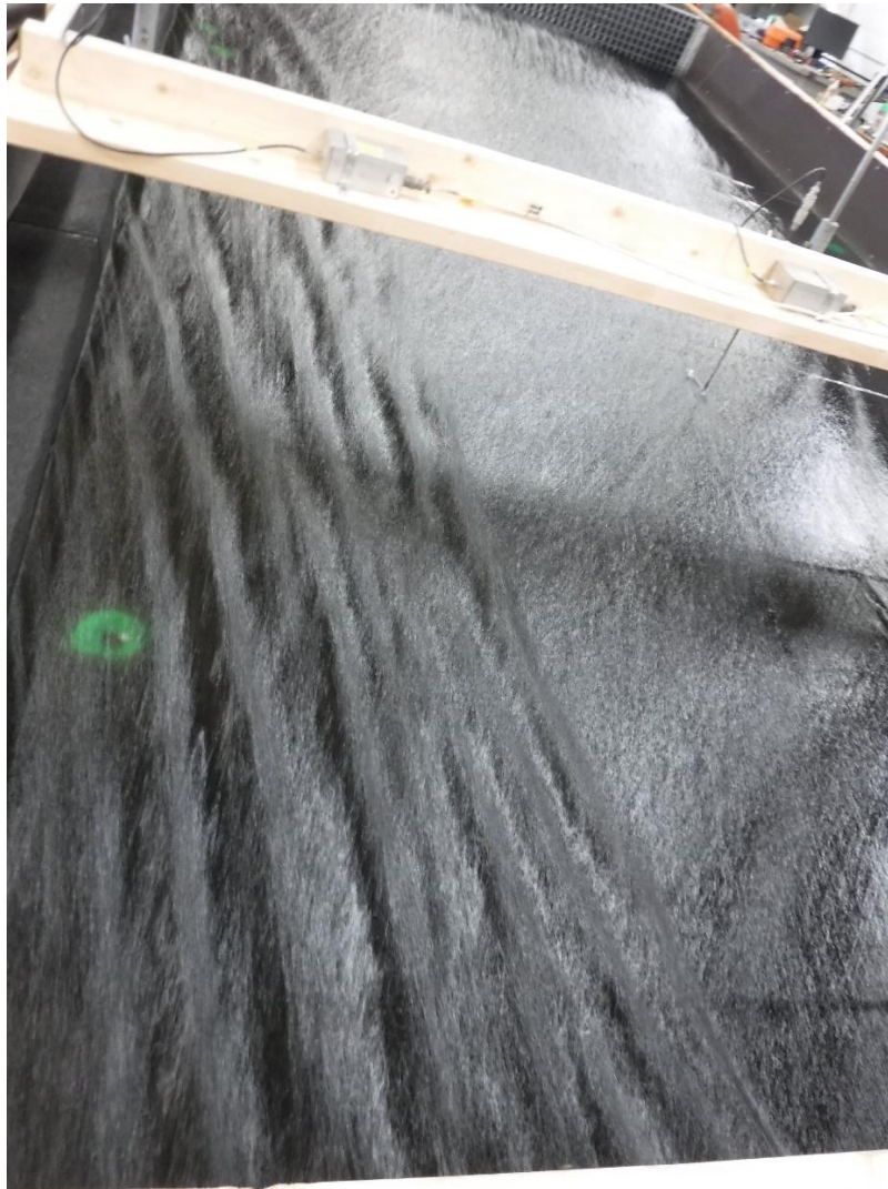
Figure 30. Standing waves forming on the roadway for test 2021-5-14_test034, Pump setting of 6 PSI and valve at 50%.
