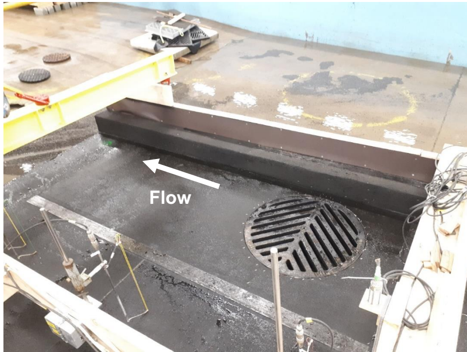
Figure 10. Single round cover with herringbone pattern (cover 1)
