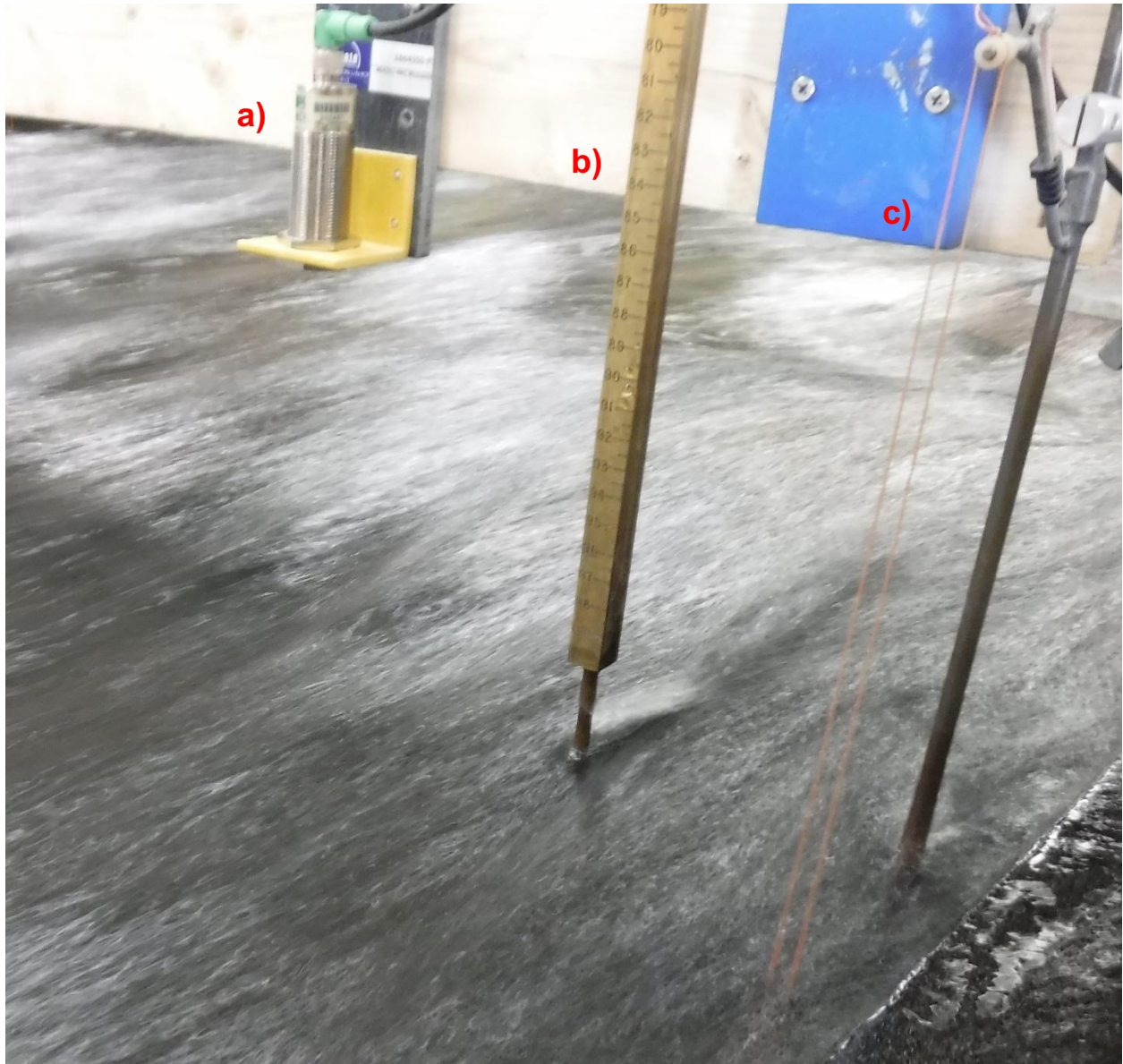
Figure 4. Water level gauges; a) UltraLab ULS, b) point gauge and c) capacitance wire gauge.
