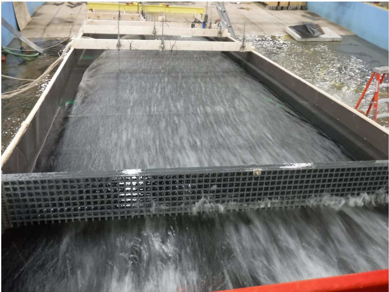
Figure 2. Model roadway image with flow straightener
