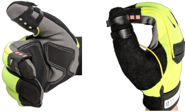
Figure 12. RFID Tip-Tap device on a glove with smooth pads. Pressing thumb and index contacts together connects two RFID chips in series, and two flexible core wires work as a single dipole antenna.
