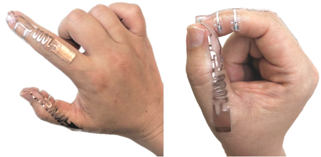
Figure 13. RFID Tip-Tap device as an on-skin tattoo. Each contact array has 3 RFID chips connected to a copper tape half-antenna shaped like half of an ALN-9740 RFID tag.
