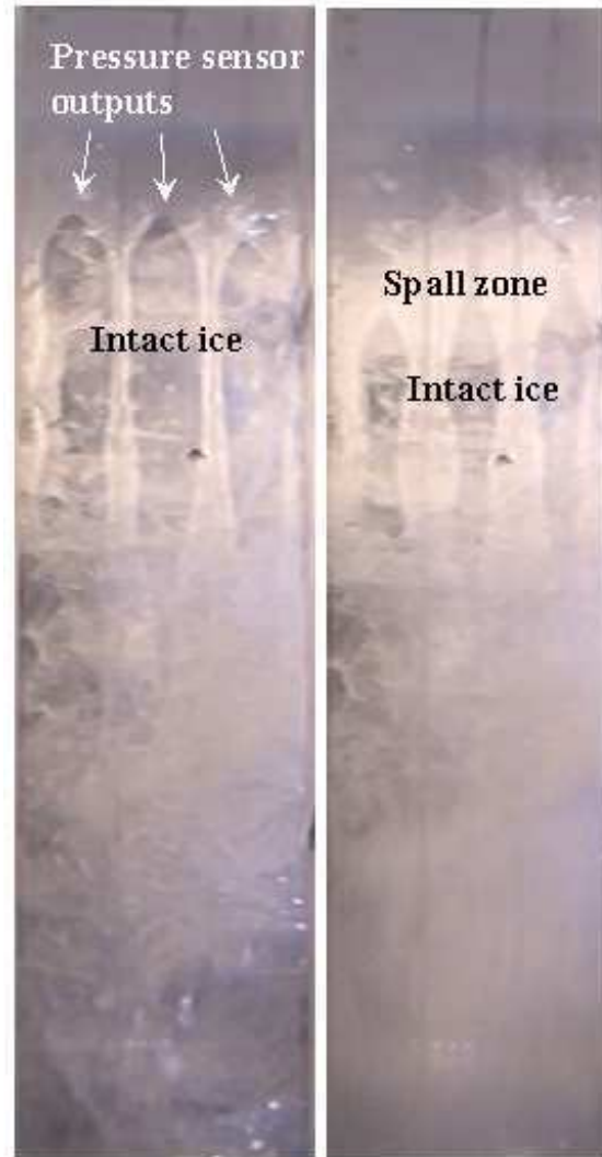
Figure 7. Images from the downward-viewing camera just before (left) and just after (right) the second spall event in Figure 6. Each image is 3 cm wide.
