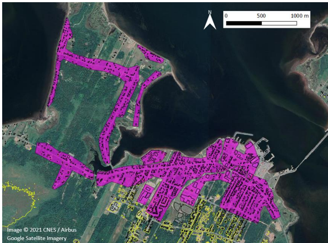
Figure 24. Example of building drag zones implemented in the communities of Shippagan and Pointe-Brûlée. Building and infrastructure footprints are outlined in black, purple polygons indicate drag zones, and the yellow line indicates the elevation contour coinciding with 4m CGVD2013.
