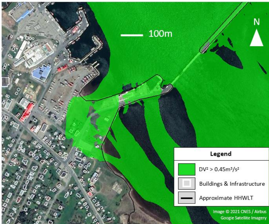
Figure 46. Momentum flux exceeding 0.45\text{m}^3/\text{s}^2 for the 1% AEP event near the Route 113 causeway connecting Shippagan to Savoy Landing.
