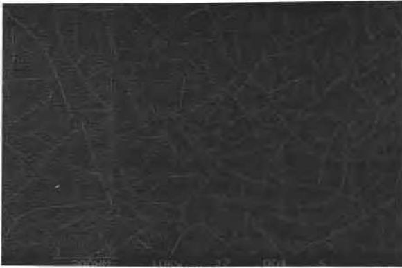
Fig. 5. Exposed surface of polycarbonate sheet protected with a surfacing film (PC-P) weathered at 0^\circ for 10 years.
