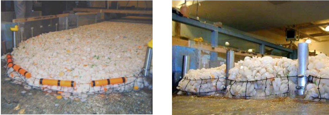
Figure 8: Two structures were tested in a laboratory. Left) A boom attached to two piers, with a net below it. Right) Nets between piers. Both are meant to retain ice runs. From Morse [24], with permission from the publisher.
