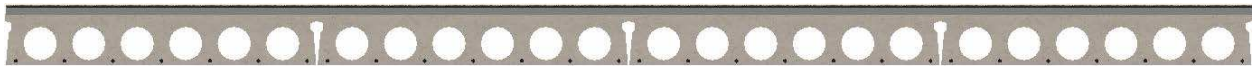
Figure 4: Floor of 203 mm thick precast concrete hollowcore slabs with a 25.4 mm underlayment poured directly on the floor. An 8 mm underpad and a 6 mm carpet were installed on the underlayment.
