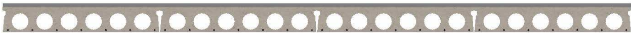
Figure 3: Floor of 203 mm thick precast concrete hollowcore slabs with a 25.4 mm underlayment poured directly on the floor.
