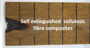
Self extinguished cellulosic fibre composites
