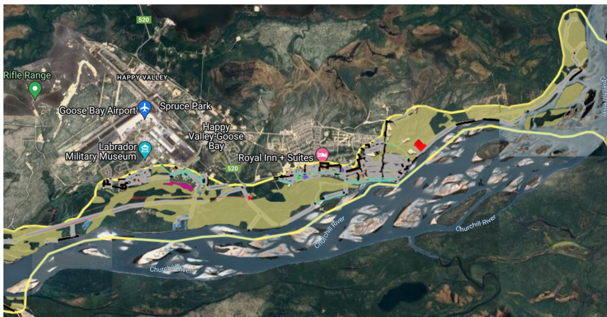
Figure 11. Inundation module of the Churchill River Flood Forecasting System with allowable inundation extent where depths and probabilities can be indicated.
