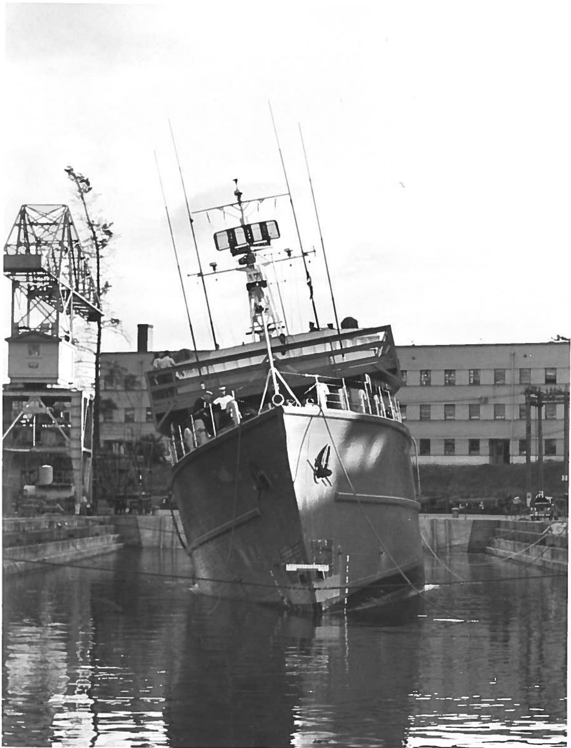
FIG. 3 BOW VIEW — ROLLING SHIP IN N-S DRY DOCK
