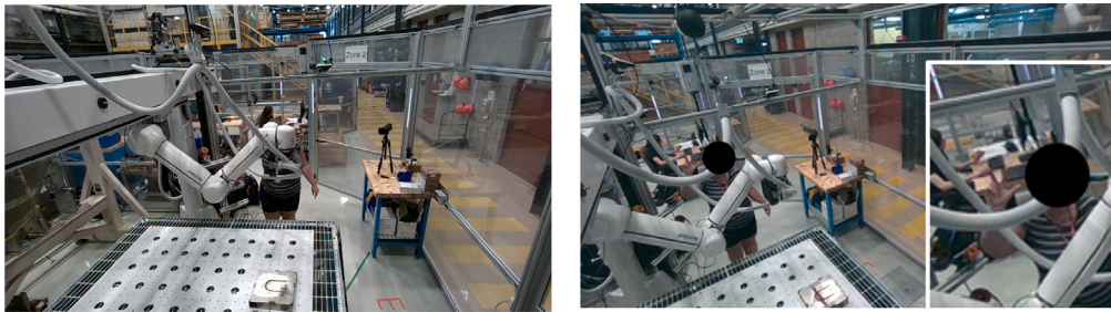
Fig. 12. Illustration of how the multi-camera configuration can correct occlusion problems. In the image on the left we are able to locate the hand but not recognize the gesture, whereas in the image on the right, obtained from another point of view, we can recognize gesture three.
