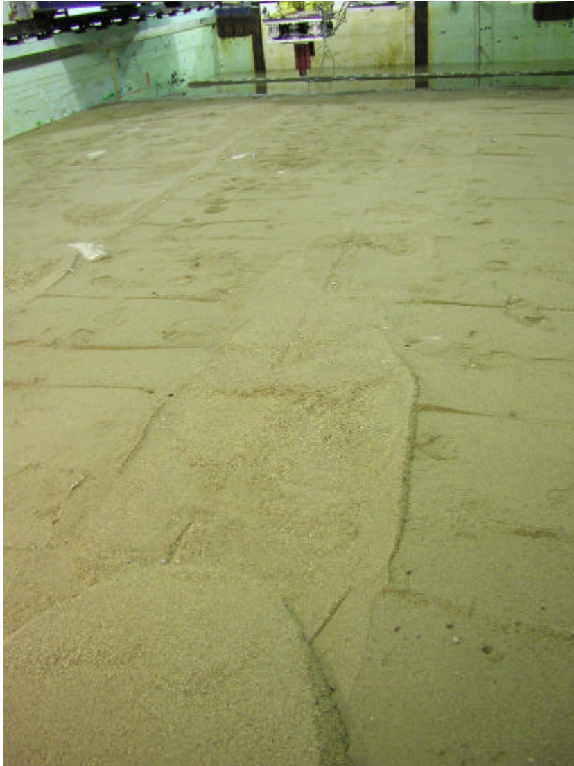
Figure 22 Photo showing the chattering effect after the ice model rode up on top of the seabed material.
