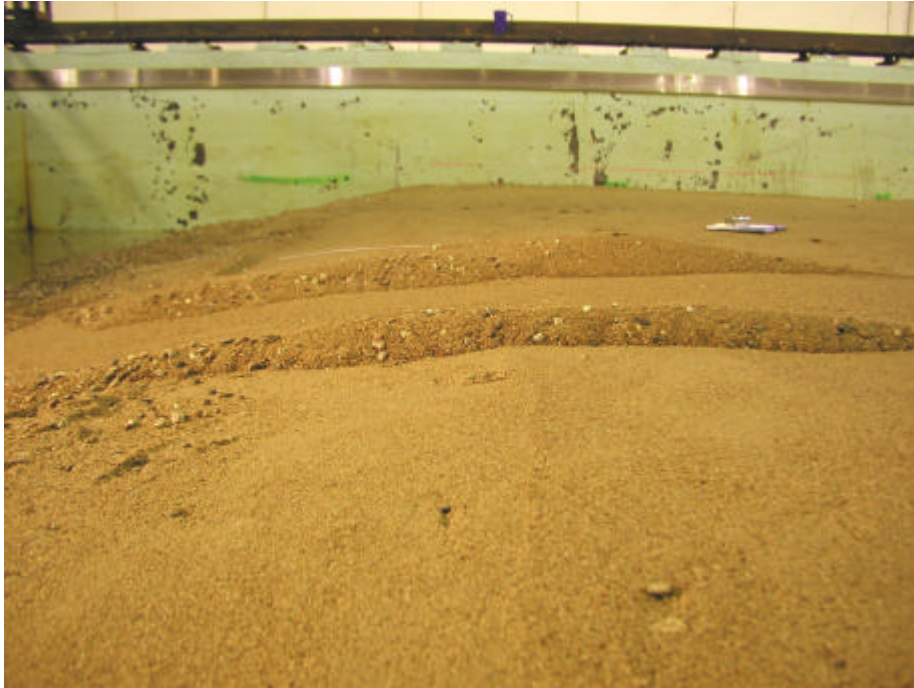
Figure 21 Side view of Scour2_007 profile. The direction of motion of the iceberg was from left to right in the photograph.
