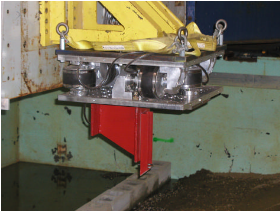
Figure 9 Dynamometer mounted on main carriage, with the steel bracket that was used to support the chain
