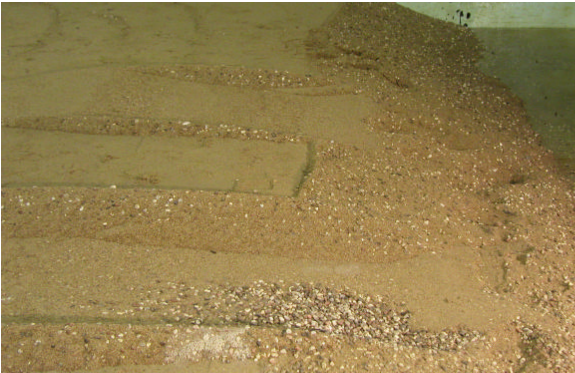
Figure 4 Photo showing the sand and gravel mixed seabed, after two tests.
