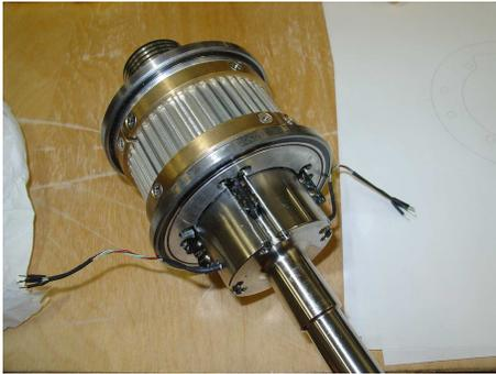
Figure 2. Drive gear subassembly.
