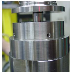
Figure 4a. Range of gap distance settings (max gap)
