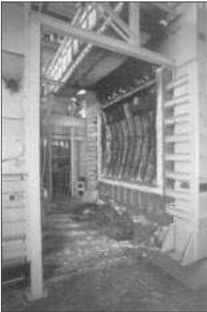
Figure 1. A gypsum board wall assembly undergoing testing in IRC's propane-fired vertical furnace.
