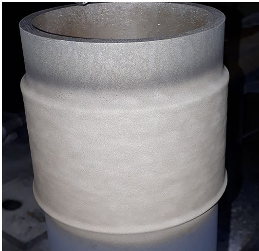
Fig. 7 Photograph of Ti-6Al-4V buildup of approximately 5 mm thickness on 114-mm-diameter steel mandrel
