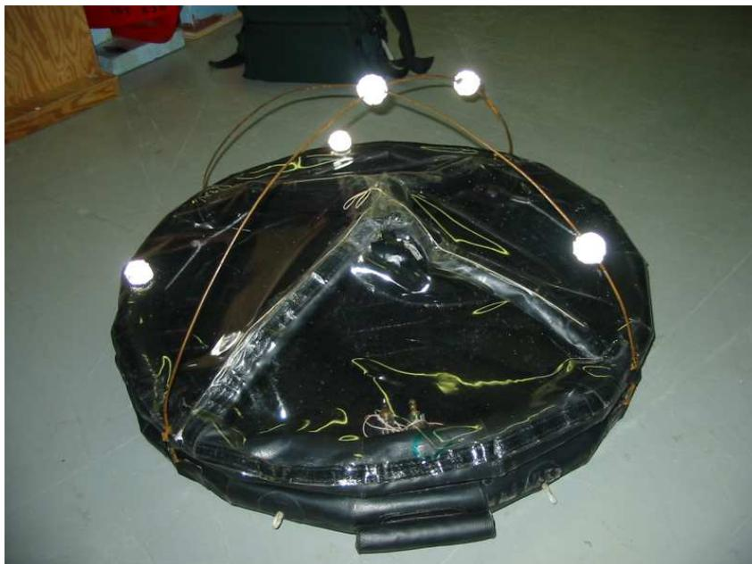
Figure 3.6: Model IOT 722 of a 42 person life raft.
