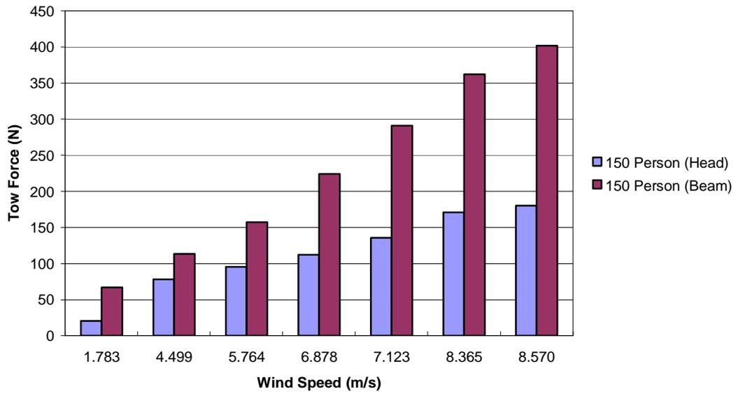
Figure 6.4: Mean tow loads for the full scale 150 person life raft, head and beam on to the wind field, across varying wind speeds
