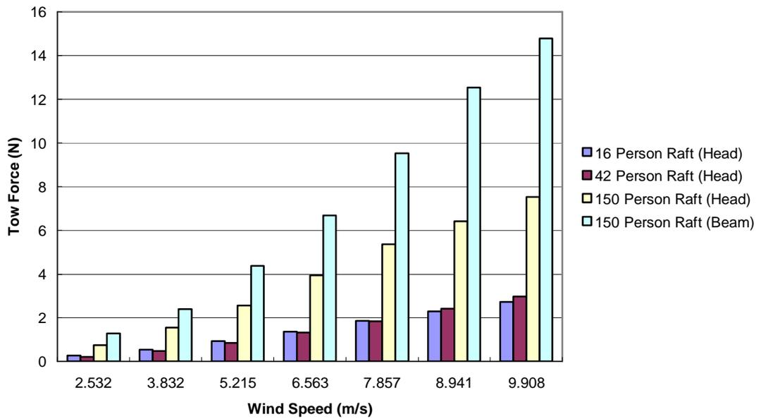
Figure 6.5: Mean tow loads for the model scale rafts across varying wind speeds.
