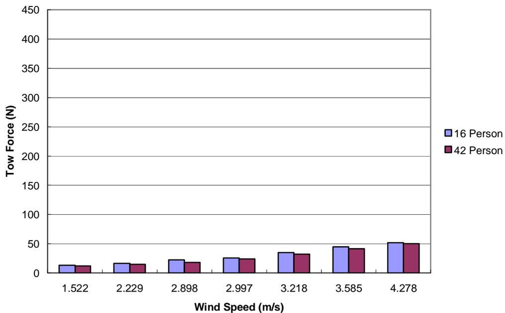
Figure 6.3: Mean tow loads for the full scale 16 and 42 person life rafts across varying wind speeds.
