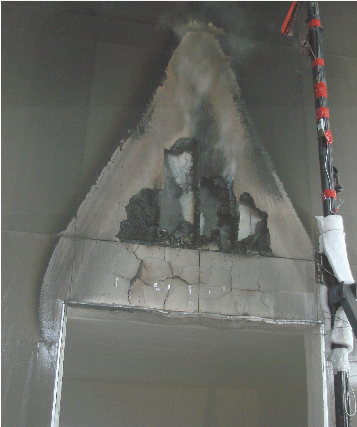
Figure 13. Wall Assembly after Fire Exposure.
