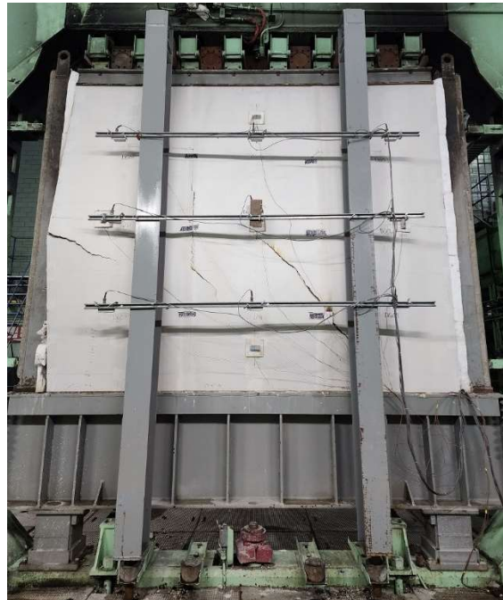
Figure 12. Fire test specimens' failure
