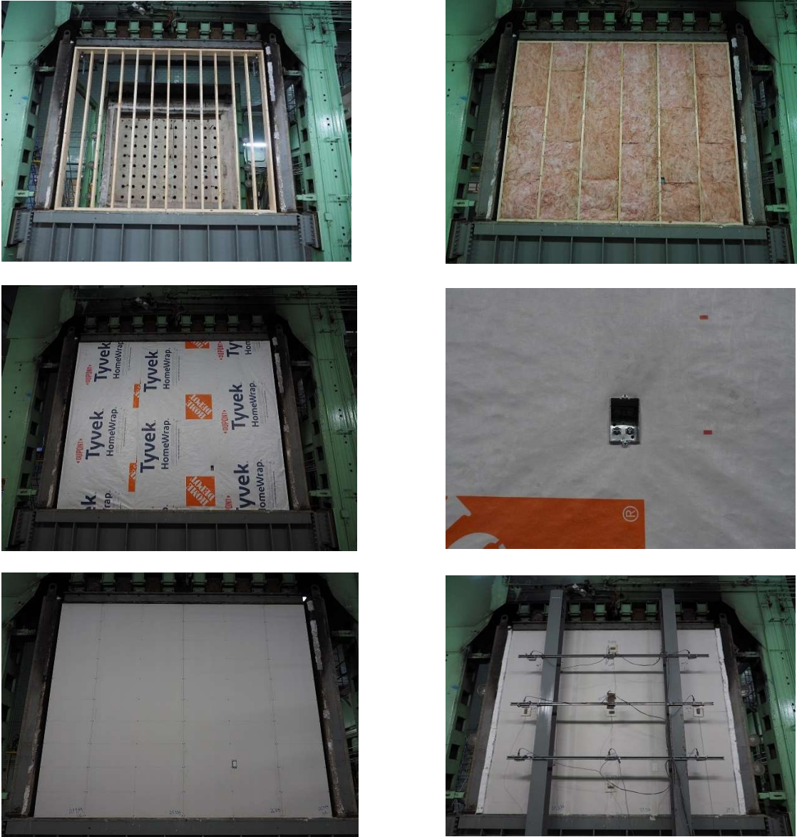
Figure 37. Specimen F2 construction photos
