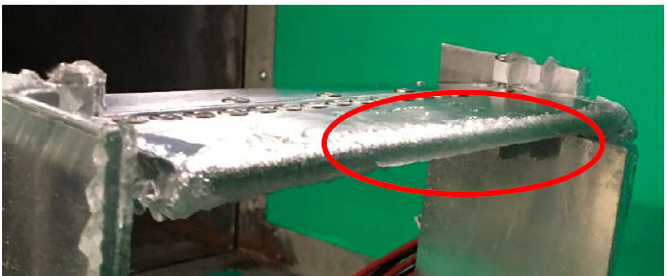
Figure 10. Delamination at 352 V pp for mode 5, repetition 2, with all piezoelectric actuators excited in phase.
