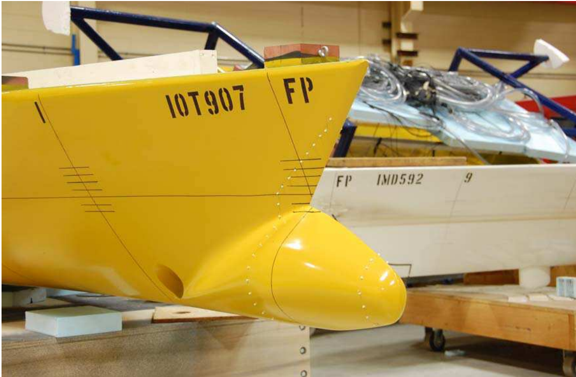
Figure 6 - IOT907 Turbulence Stimulation
